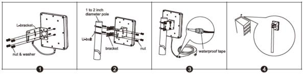
**Note:** Wrap waterproof tape around the connectors between outdoor antenna and feeder line to avoid water or other kinds of damage.
