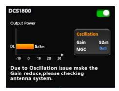
Repeater system will strictly check Self-oscillation degree for all of sub-band and firstly will show abnormal status (Orange) in Menu page, ISO and ALC function would auto generate and if user enter into the soft Self-oscillation sub-band, user could check more details about Self-oscillation with recommend info.
