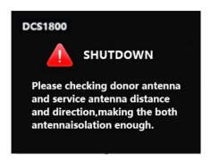
if not working and Self-oscillation get seriously, which overcome ISO and ALC function address range (ALC≥42dB, ISO≥42dB), the Sub-band (with Self-oscillation) would be auto-shutdown ass above message, which shows shutdown status (red) for this Sub-band in Menu Page, to protect Base Station wouldn't get interference.
