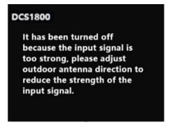
This system auto-generate message caused by excessively strong signals from cell tower, referring to below troubleshooting sections.
