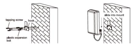
If you have an indoor Omni ceiling antenna, the best place to install it is the center of your house. Install Omni ceiling antenna as shown in the graph below.
